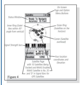
It normally takes a couple of minutes for the GPS receiver to "home-in" on the satellites, and to determine a location. Initially, the status window may read: *Wait...tracking satellites*. The GPS receiver can not be used until it reads: *Ready to Navigate*.
